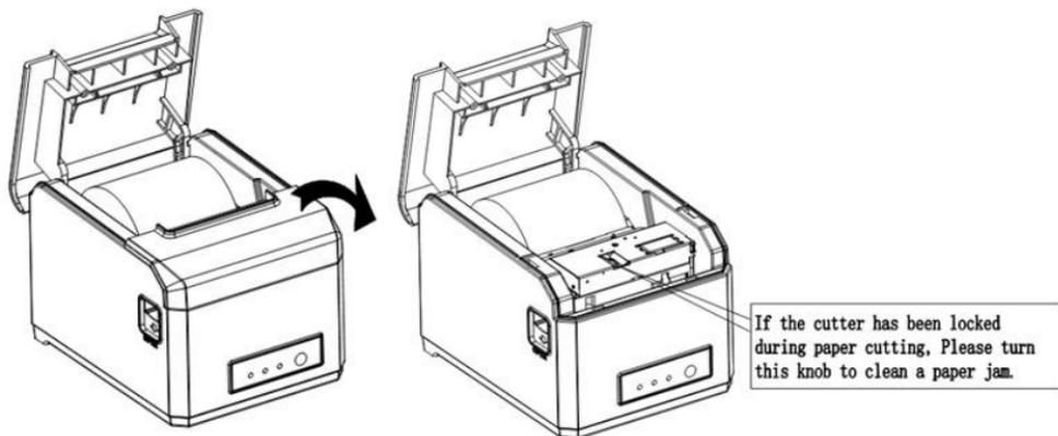
Note: do not force open the cover, as to avoid unrecoverable damage to the print head and the cutter.
